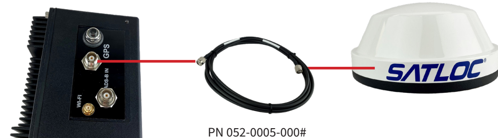
Figure 3-8: Connect A21 antenna cable to Falcon CPU and A21 antenna
