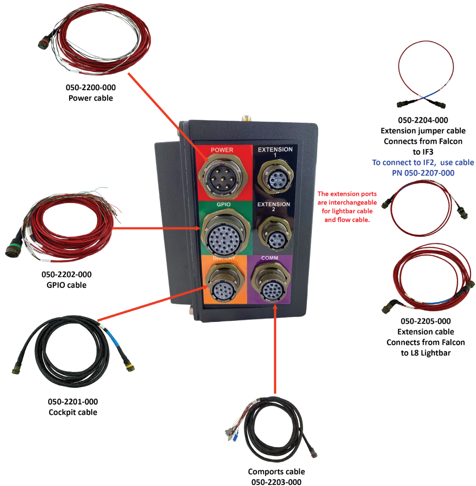
Foto 3-1: Connections to Front of Falcon
