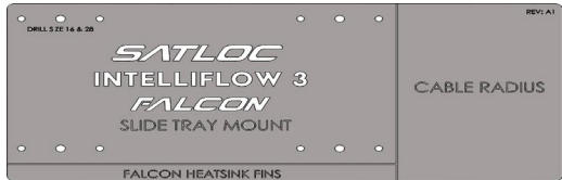
Figure 2-1: PN 601-1313-000 (Optional, Available for Purchase) Mounting Layout Template for Falcon/IF3 Rack Mount (See Appendix C for dimensions reference.)
