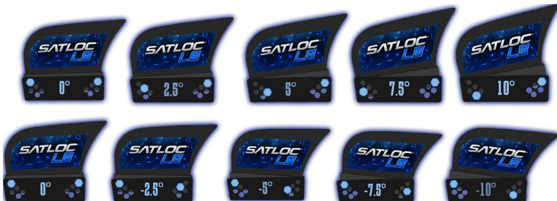
Figure 2-4: Tilting Angles of L8 Lightbar
