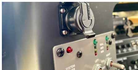
Figure 2-3: Install Image of Optional USB Port
