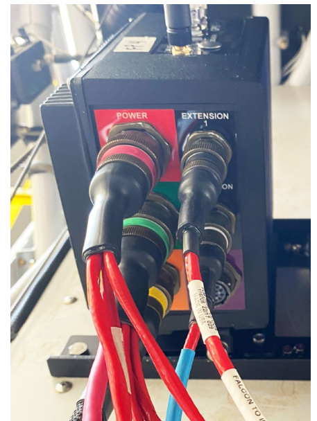
Figure 3-2: Install Image of Connections to Front of Falcon
