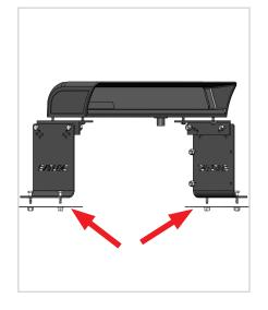
Using hardware F, secure the lightbar to the aircraft. If required, use the backing plates on the underside of the mounting surface for additional reinforcement (these provide additional support to prevent the bolts from pulling through the surface under vibration).
