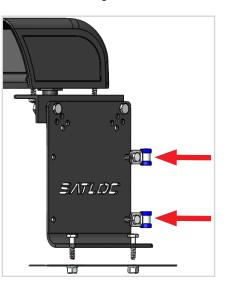
Connect cable to the bottom of the lightbar. Using hardware **G**, attach the cable to the lightbar. Be careful not to make any sharp turns or bends.
